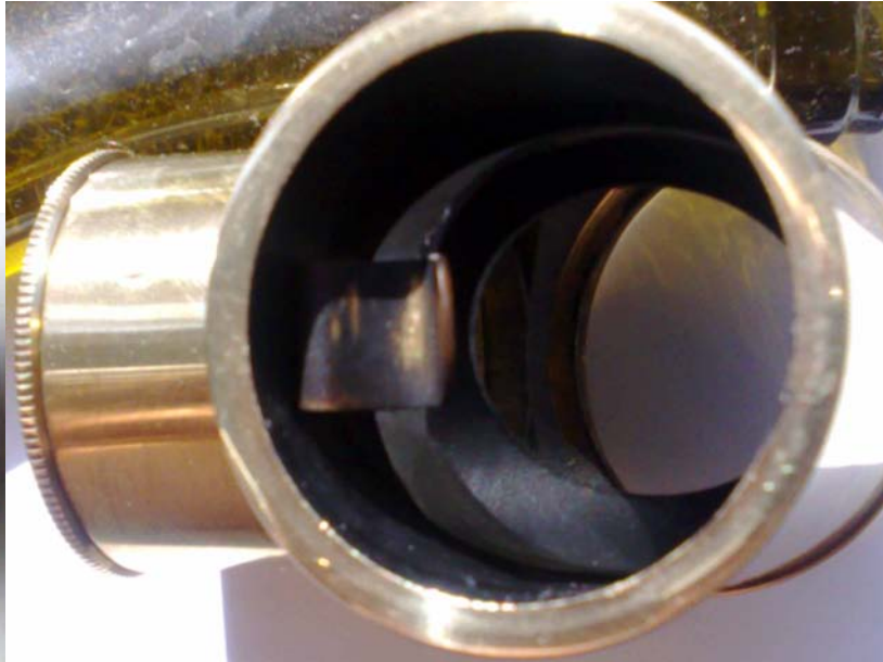
BRASS WATSON SUN DIAGONAL c1890. A Herschel Wedge solar prism, originally suggested by John Herschel c1830.
