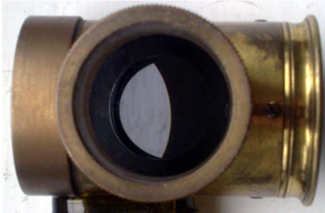
BRASS WATSON SUN DIAGONAL c1890. A Herschel Wedge solar prism, originally suggested by John Herschel c1830.
